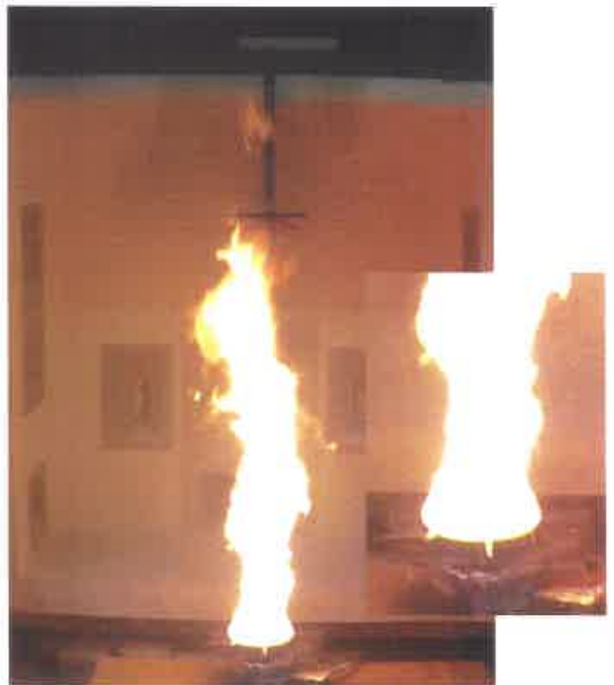
Photo: 7 min 54 sec of video: P17-094-4: Enlargement of flames and ejection of burning material after firefighting (full view and detail).
