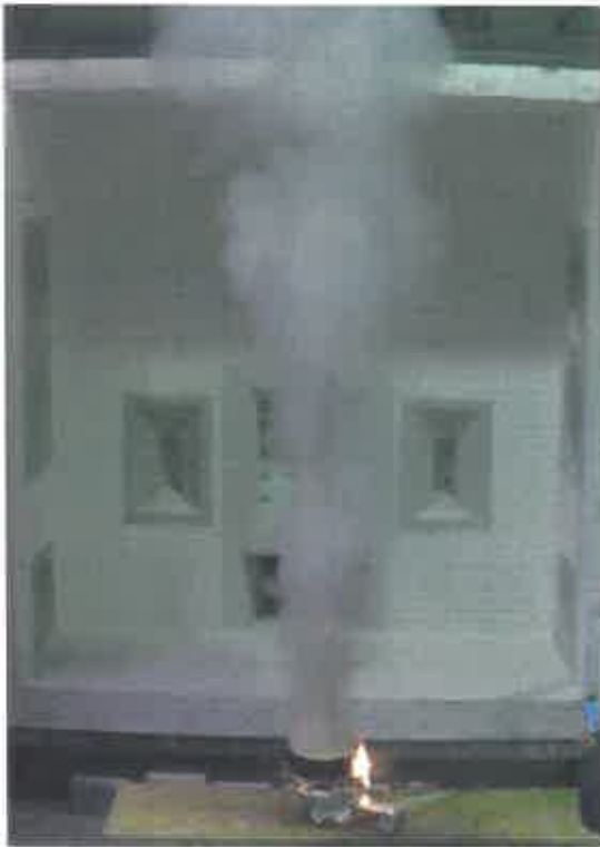
Photo: 9 min 34 sec of video: P17-094-2: Extinguishment of the fire 21 s after commencement of firefighting.
