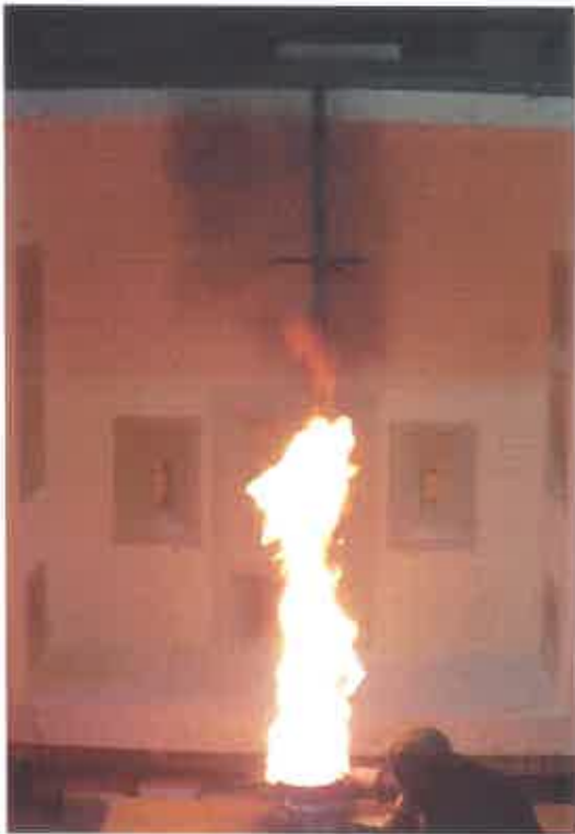
Photo: 7 min 51 sec of video: P17-094-4: Commencement of firefighting 121 seconds after the start of the fire.
